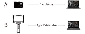
When operating the copy, if the machine is not connected to the computer, please restart the machine or plug and unplug the Type-C data line. Do not plug and unplug the Type-C data cable during the data transmission process, which will cause the data transmission to fail.
